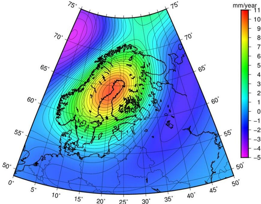
Gridded vertical geometric displacement rate
