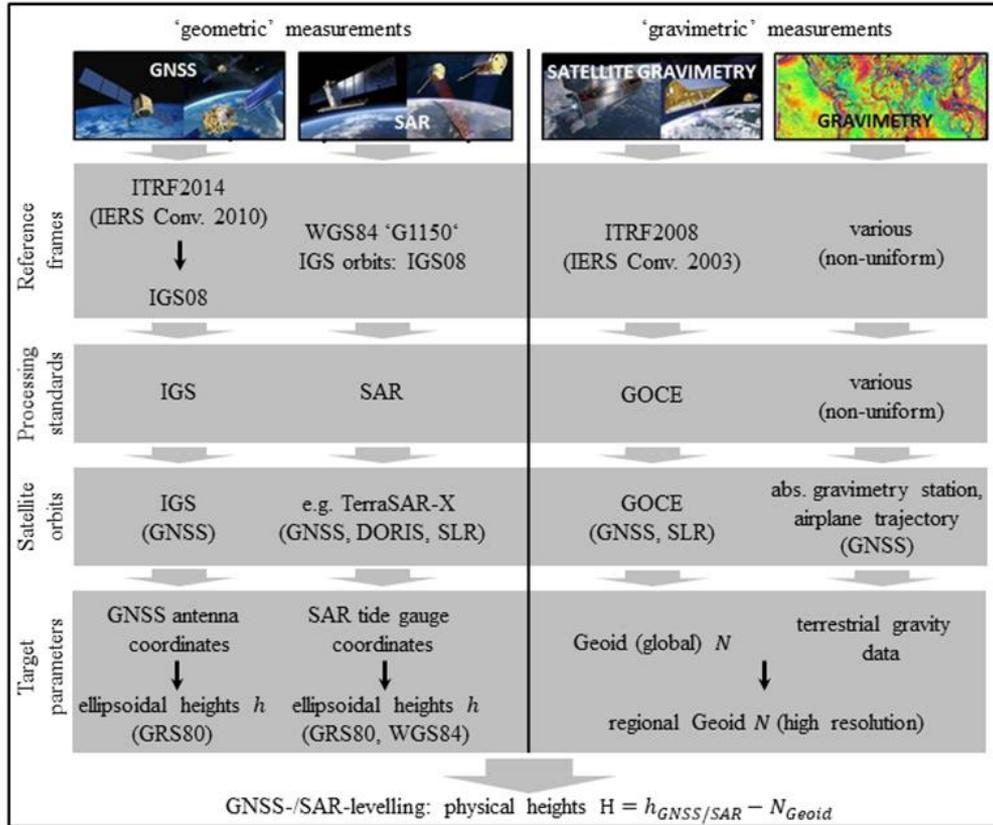
Simplified scheme for the determination of ellipsoidal heights from the geodetic SAR technique and GNSS (left) and the determination of physical heights referring to a common physical reference surface based on GOCE and terrestrial/airborne data (right).
