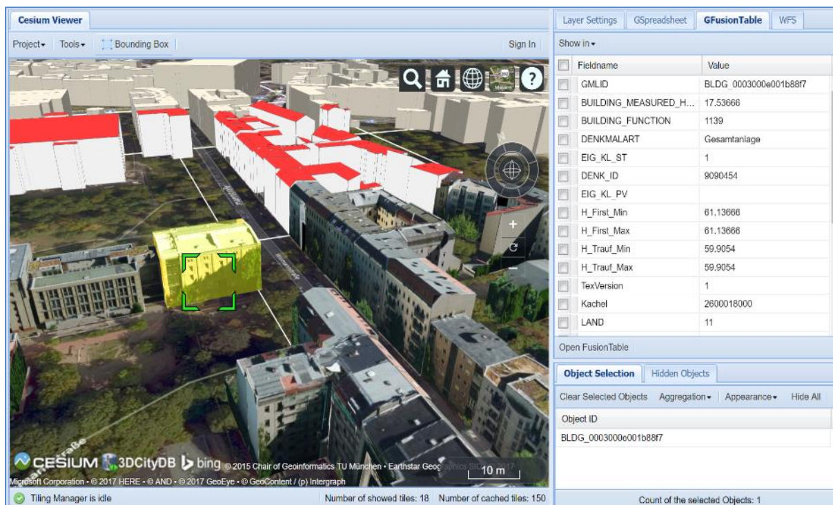
Figure 99: Example of visualizing 3D city model of Berlin on the 3D web client
