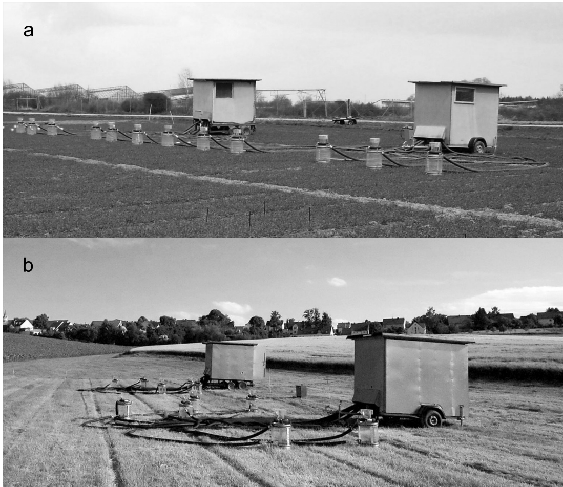
Figure 2.3: NH 3 measurement system installed on winter wheat (a) and grassland (b) experimental site Dürnast in the years 2004 (a) and 2008 (b).
