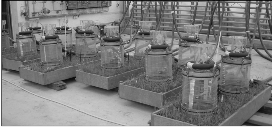
Figure 2.5: \text{NH}_3 measurement system installed on trays in the greenhouse.
