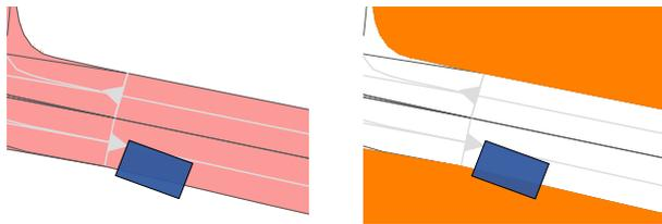
(a) Enclosure checking: Is the blue vehicle enclosed in the red allowed region? ( $\mathcal{E} \subseteq \mathcal{A}$ ?)
