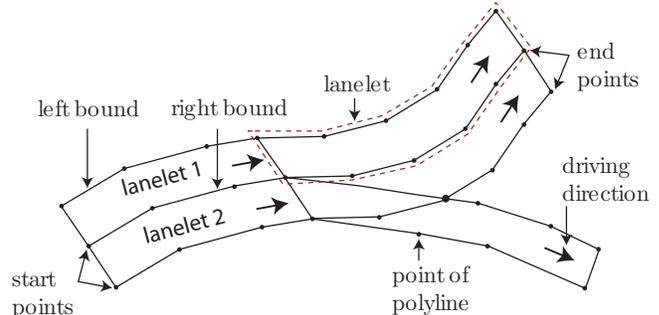
Fig. 2: Road network composed of lanelets.
