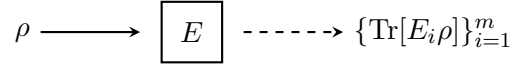
Figure 2.1: Measurement of a system in quantum state \rho \in \mathcal{D}_d represented by a POVM E \in \mathcal{E}_{d,m} . The measurement outcome i is observed with probability \text{Tr}[E_i \rho] .
