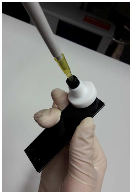
FIGURE 3.7: Direct injection of the reaction mixture in the microarray flow channel by using an housemade adapter.
