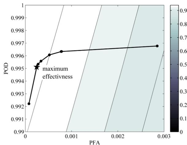
*Figure 11: The resulting Receiver Operator Characteristic ROC curve of the Illgraben alarm system, overlaid on the effectiveness.*
