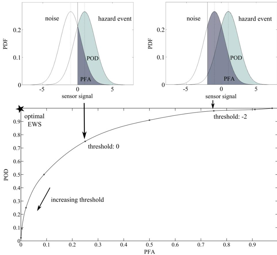
**Fig.1.** Conditional Probability Density Functions (PDFs) representing noise and a hazard event and the Probability of Detection (POD) and Probability of False Alarms (PFA) for two different thresholds (upper part). Correlated Receiver Operator Characteristics (ROC) curve for varying thresholds and the optimal performance of an EWS (lower part).
