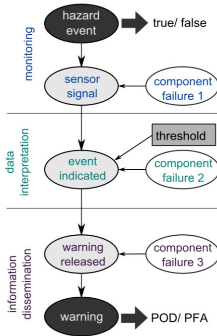
**Fig. 4.** Schematic framework of a Bayesian Network (BN) to model the reliability in terms of Probability of Detection (POD) and Probability of False Alarms (PFA) for alarm systems.
