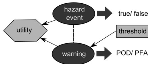
**Fig.5.** Schematic Decision Graph (DG) to identify the optimal threshold combination that maximizes the alarm system effectiveness.
