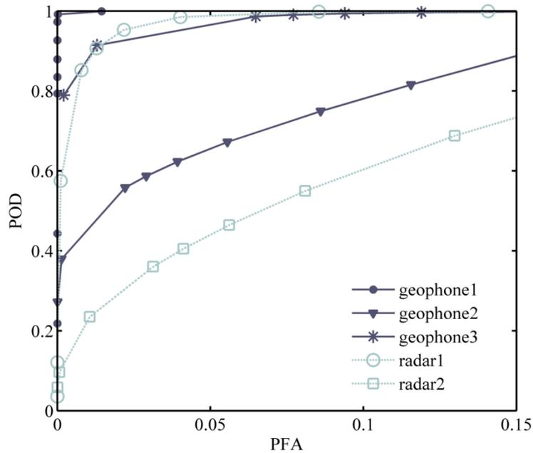
**Fig. 9.** Receiver Operator Characteristic ROC curves illustrate the reliability of sensors for nine predefined thresholds. The highest threshold is represented by operation points left. Geophone 1 shows the best performance.
