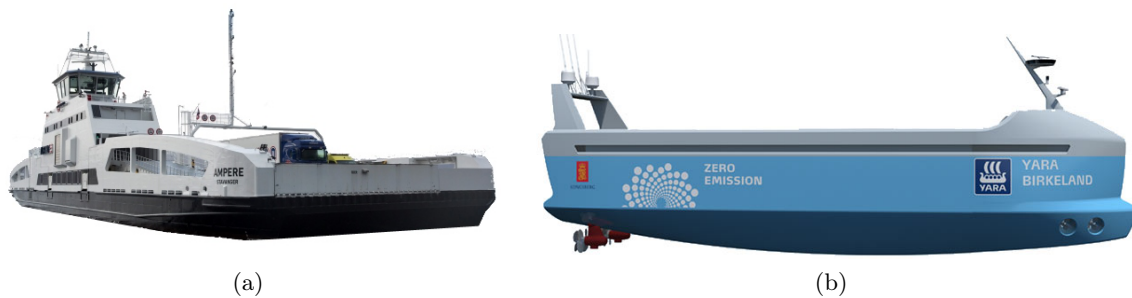
Figure 1.2: Examples for pure electric ship propulsion systems. The already operating electric ferry “Amper” is displayed in (a) [135] and the container ship concept “YARA Birkeland” in (b) [76].
