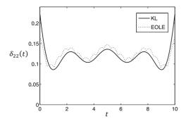
Figure 2. Point-wise variance error  $\delta_{22}(t)$  for the multivariate KL and EOLE methods with m = 6.
