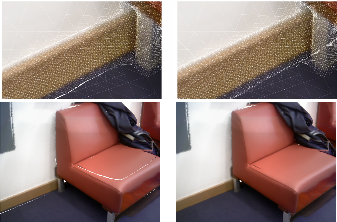
Figure 4.9: Joining of GPT mesh with planar segment triangulations. Left shows unjoined segments and right shows segments joined with interpolated boundary vertices.
