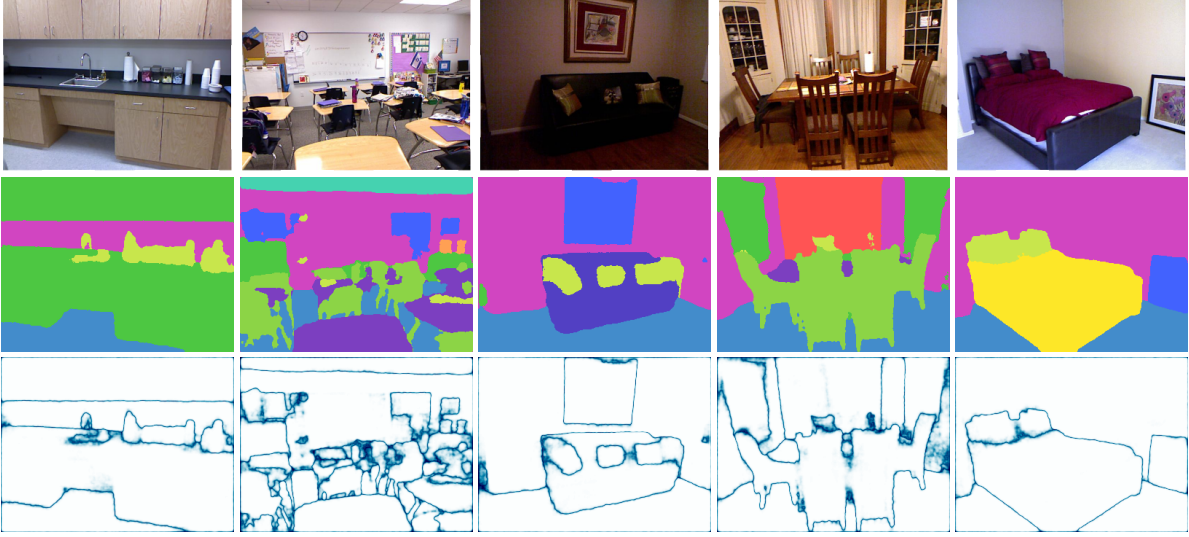
Figure 12.2: The uncertainty of CNNs semantic segmentation prediction (color code: the uncertainty increases from low to high corresponds to color from white to dark).
