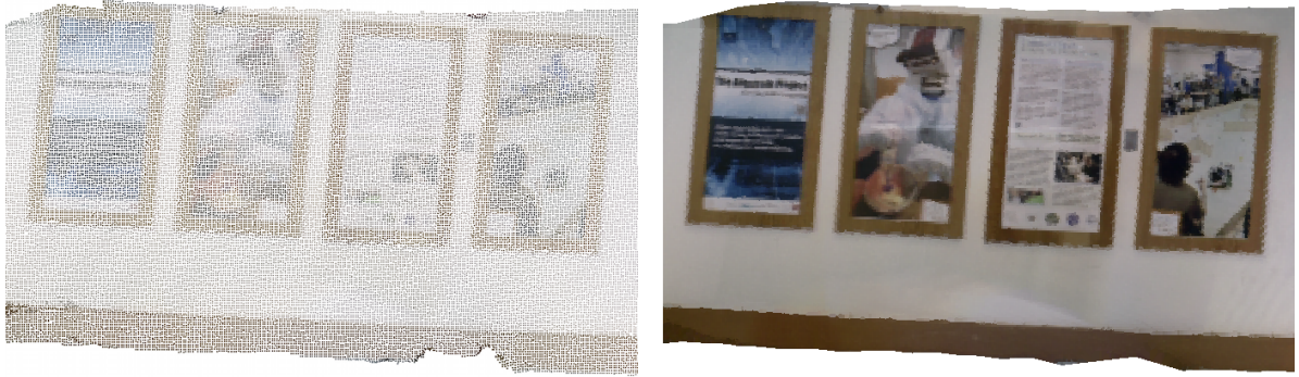
Figure 4.6: Texture generation: (left) plane segment from a colored point cloud; (right) generated texture.
