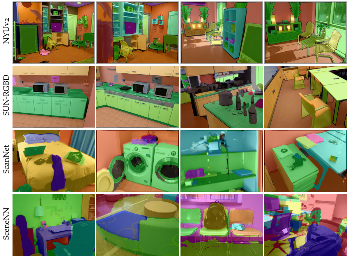
Figure 9.2: The limitations of state-of-art RGB-D annotations. NYUv2 (Silberman et al. 2012) and SUN-RGBD (Song et al. 2015) use polygon-based annotation, which leads to label inconsistency between multiple viewpoints. ScanNet (Dai et al. 2017a) and SceneNN (Nguyen et al. 2017) proposed segment-based mesh annotations, where objects are not accurately extracted and details are lost. In both scenarios, 2D labels are offset with respect to the actual object boundary.
