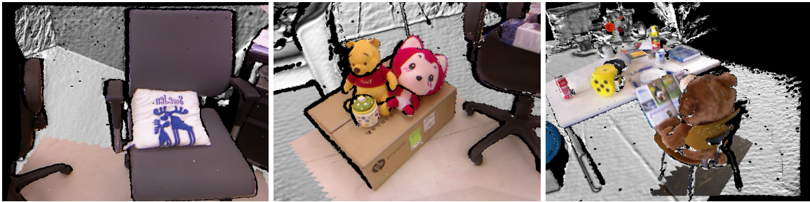
Figure 10.8: Synthetic view by ray casting the volumes. The colored and gray scale pixels are obtained from the constructor and the helper, respectively. Notice how the helper volume fills in the missing pixels to assist tracking.
