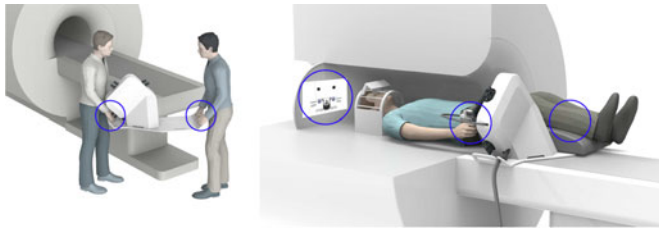
Fig. 8. Main user interfaces of the MR-Octo for scientists (left) and subjects (right).
