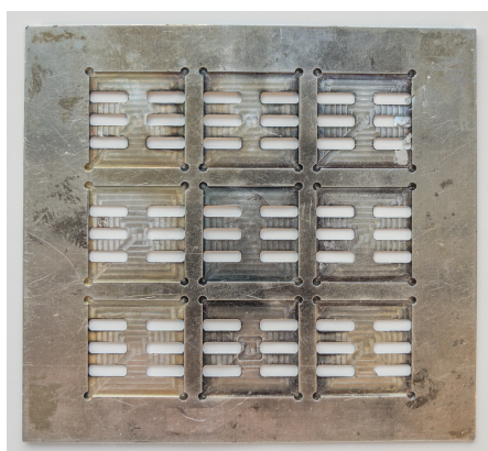
Figure 3.6: Shadow mask used for the evaporated top electrodes. Each sample is covered with six fingers, which have a width of 3 mm.
