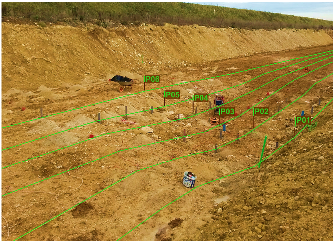
Fig. 28: Photograph of the 2.5D ERT survey layout, with six 60 m long profiles (P01 – P06, 0.75 m inter-electrode spacing, 45 m maximum field layout, 1.5 m line spacing) oriented perpendicular to the long axis of an oval-shaped collapse doline and the most prominent voids (viewing direction from west/Stuttgart to east/Ulm).
