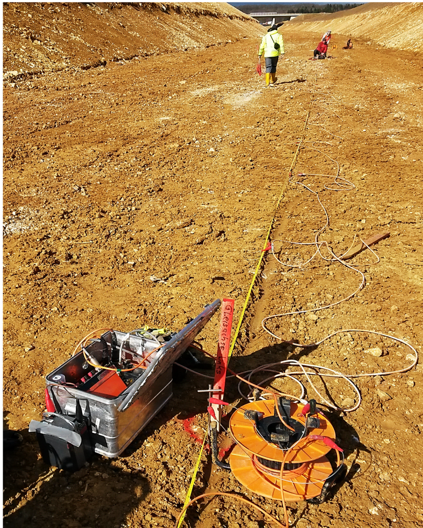
Fig. 20: Photograph of the 2D ERT survey layout, with one 150 m long profile (2.5 m inter-electrode spacing, 150 m maximum field layout) along the northeastern line track (direction Ulm to Stuttgart).
