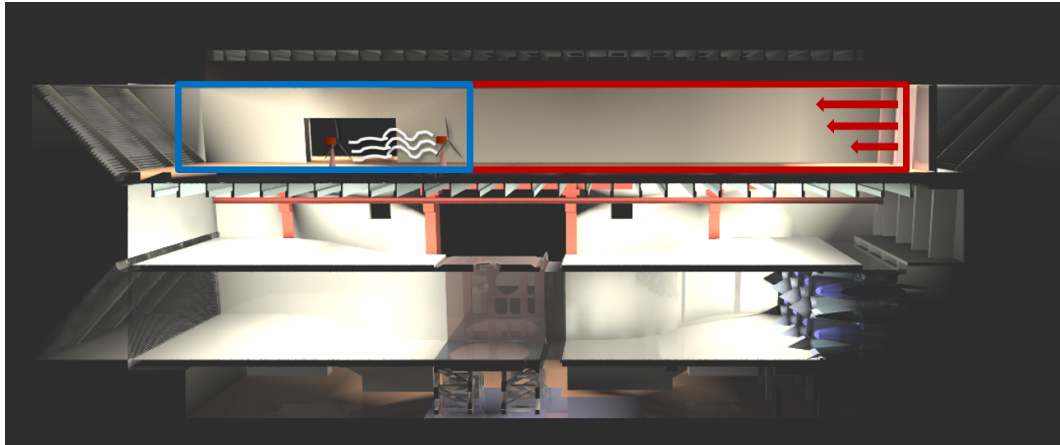
Figure 3.1: Picture for the sectional view of the boundary layer wind tunnel at Politecnico di Milano (POLIMI) [57].
