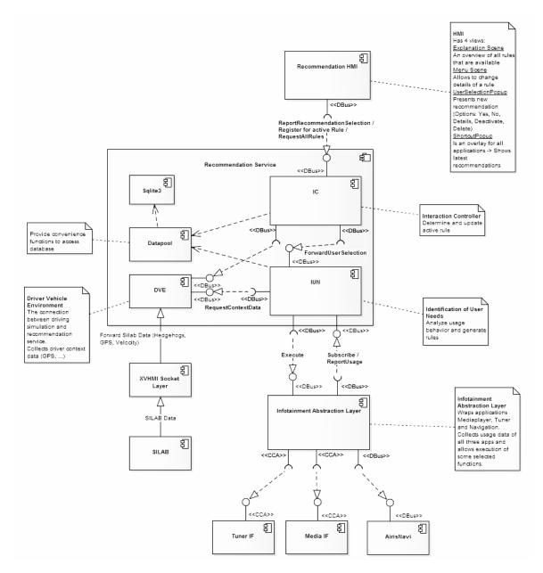
*Figure 7-8.:* Components and interfaces of the adaptive recommendation service integrated in the infotainment system of the pre-development platform of Bosch.
