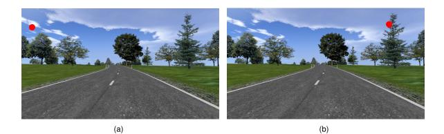
*Figure 8-5.:* Screenshots of the driving simulation showing a stimulus of the DRT on the left (a) and right side (b) of the road. Both pictures are examples for possible positions of the DRT stimuli.
