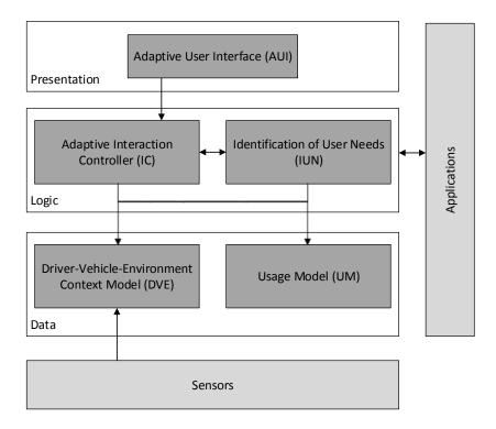
*Figure 5-2.:* Blog diagram of the reference architecture of an adaptive recommendation service based on a three-tier-architecture
