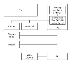
*Figure 8-3.:* Involved technical components: driving simulator with pedals and steering wheel, head unit and cluster, connection tool and driving simulation software running on a PC, and TV presenting the driving simulation.
