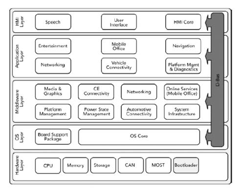
*Figure 3-4.:* Infotainment systems can be represented as layered architecture consisting of five different layers and a communication component for communication between the layers (Kocher and Kleiner, 2008).
