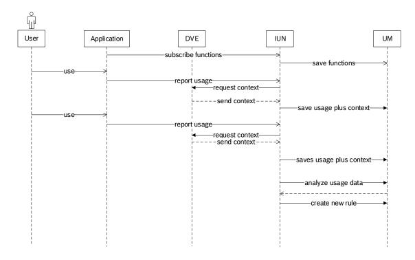
*Figure 5-4.:* Components and interfaces of an adaptive recommendation service are shown according to the process to learn the needs of a user applicable to the context.
