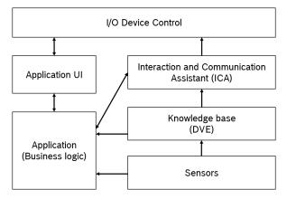
*Figure 3-5.:* The overall HMI architecture in the vehicle is a central component that coordinates all input and output from and to the user. The structure of an overall HMI architecture according to Amditis et al. (2010) is shown.
