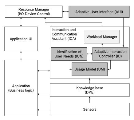
*Figure 5-6.:* The adaptive recommendation service integrated in an overall HMI architecture that is derived from the AIDE architecture (according to Walter et al. (2015a))
