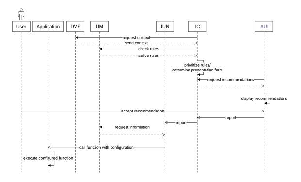
*Figure 5-5.:* Components and interfaces of an adaptive recommendation service are shown according to the process to give a recommendation to a user applicable to the context.
