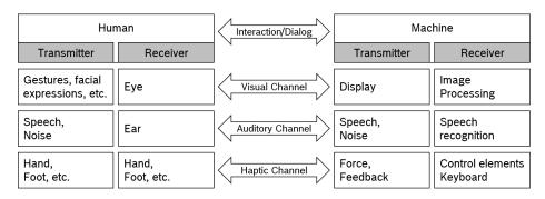
*Figure 2-2.:* In the vehicle three possible communication channels are available for communication between the vehicle occupants and the infotainment system. The three channels are the visual, haptic or auditory channel (according to Reif (2010)).
