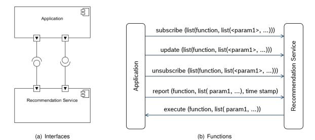
*Figure 5-3.:* Interfaces between the adaptive recommendation service and applications. Both share the roles of client and server. The adaptive recommendation service provides an interface to subscribe, update and unsubscribe functions and in addition to report usage of a function. The application provides an interface to execute an application (Walter et al., 2015a).
