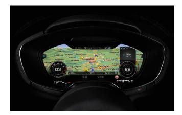
*Figure 2-8.:* On the cluster screen of the Audi TT content of the infotainment system, as for example a navigation map, is shown in addition to the usually displayed information on a cluster display as speed<sup>8</sup>.
