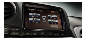
Figure 2-7.: Information about tire pressure of the vehicle's tires displayed in the 2016 Nissan GT-R<sup>7</sup>.
