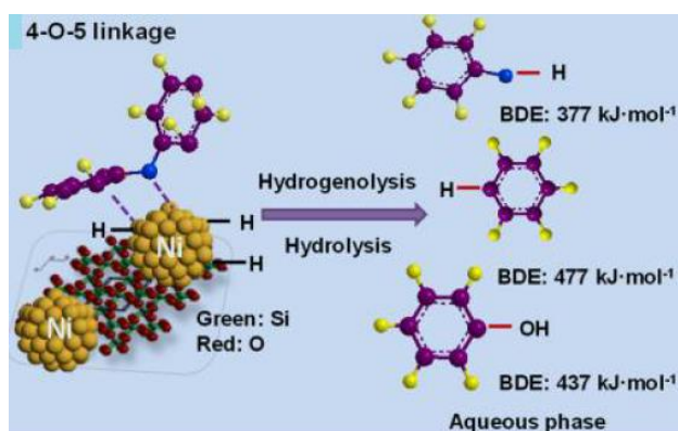
Figure 1-13. Cleavage of diphenyl ether over Ni catalyst. 44 (Reprinted and adapted with permission from reference 44. Copyright © 2012, American Chemical Society.)
