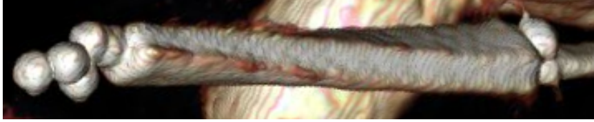
Figure 4.6.: Volume rendered C-arm CT reconstruction of fiducials equipped prototype ICE catheter. The 3D constellation of the beads is visible. The metallic beads appear larger due to partial volume effect and interpolated transfer function.
