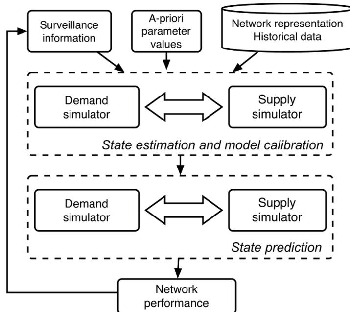
Figure 2.3: Structure of a DTA System-(Antoniou, 2004)
