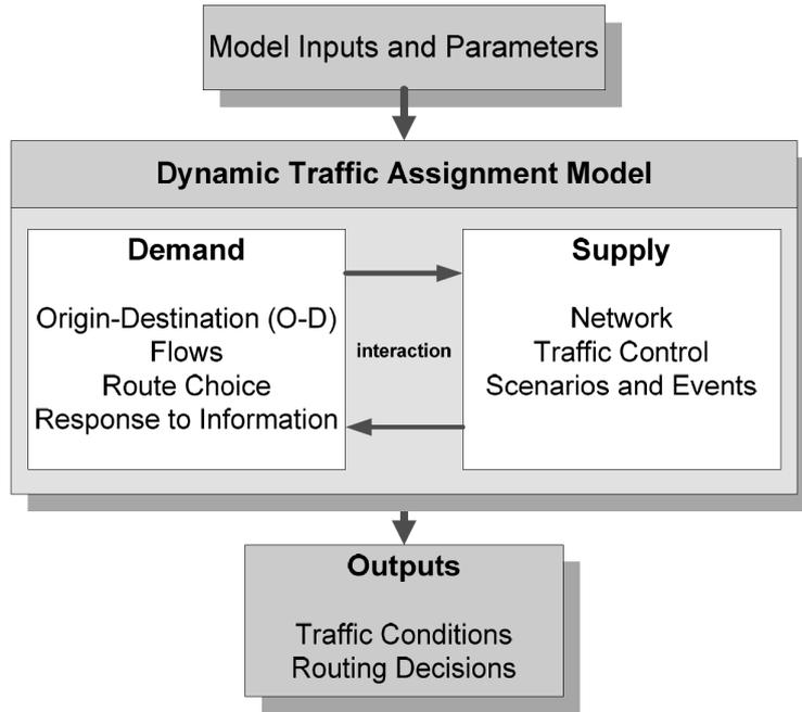
Figure 2.4: Generic interactions in a DTA model-(TRB, 2011)
