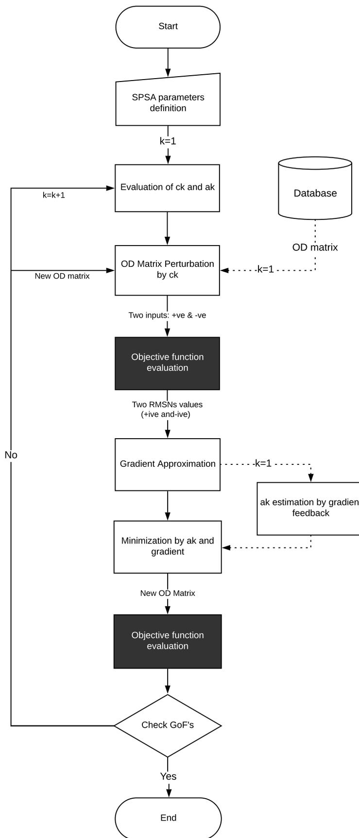
Figure 3.3: SPSA algorithm flow chart
