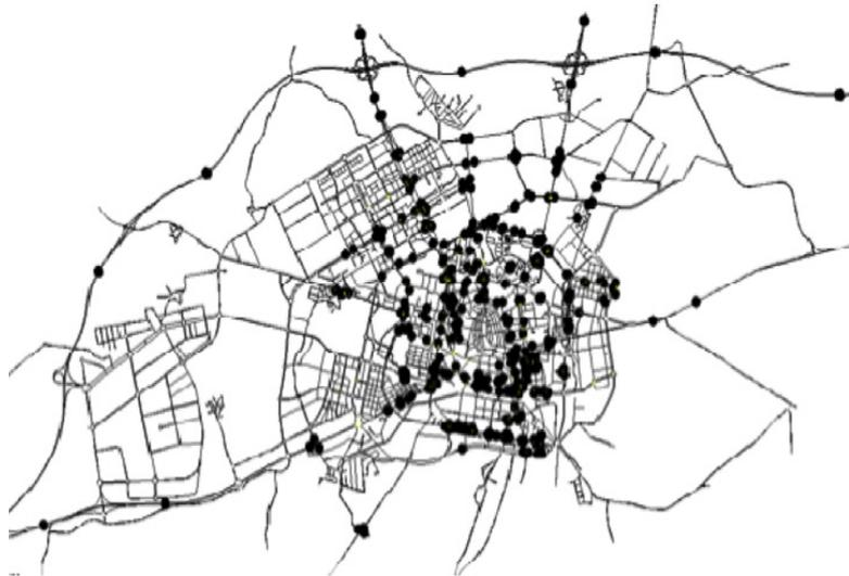
Figure 4.14: Vitoria network with loop detector locations
