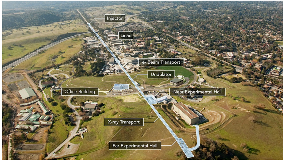
Figure 3.1: Aerial view of LCLS. The major components of LCLS are highlighted and labeled. Source: [182].
