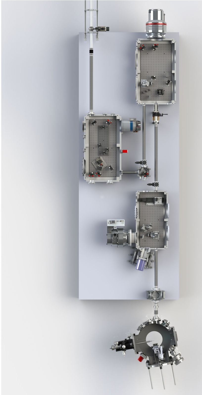
Figure 5.5: Overview of the AS101 beamline. The entire vacuum beamline AS101 in the experimental laboratory is illustrated by a detailed, comprehensive CAD model. In the depiction, the laser beam, coming out of the hollow-core fiber in the laser laboratory, enters the laboratory from the top through a wall breakthrough. Pulse compression chamber, HHG chamber and diagnostics chamber, as well as the experimental end station are clearly visible. Credit: Andreas Duensing, Technical University of Munich, Chair for Laser- and X-ray physics.
