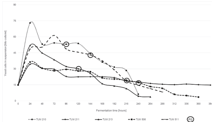
Fig. 11 Yeast cells in suspension during the main fermentation and maturing phase. The circle marks the specific final gravity of the investigated yeast strains TUM 210, TUM 211, TUM 213, TUM 506 and TUM 511
