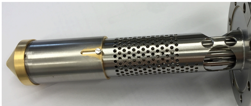
(a) Modified Feulner cone attached to the residual gas analyser
