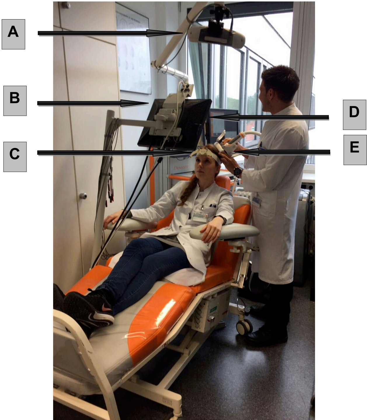
Fig. 7: The experimental setup of the Nexstim eXimia system (Nexstim Plc, Helsinki, Finland). A: Stereotactic camera for neuronavigation; B: 15-inch screen 40 inches in front of the subject for the neglect-mapping task; C: Headband with tracking system for the neuronavigation; D: 2 screens for the navigation; E: Stimulation coil;
