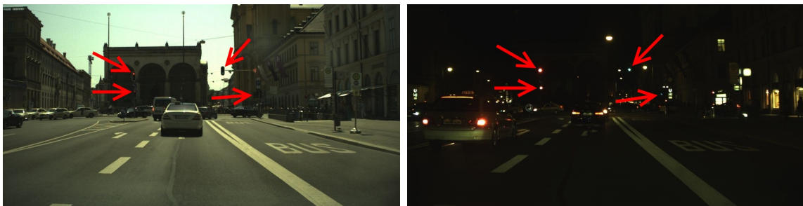
Figure 8.1: The same scene recorded on a sunny day and at night showing the challenges for a traffic light detection system that needs to operate in all conditions.
