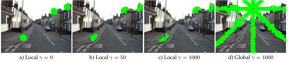
Figure 5.3: Visualization of the shapes of the geodesic neighborhoods for selected pixels (marked in black). The first 3 images show the shape of the local geodesic neighborhood for different values of \gamma , while the last image shows the global geodesic neighborhood, consisting of 8 separate ray neighborhoods.
