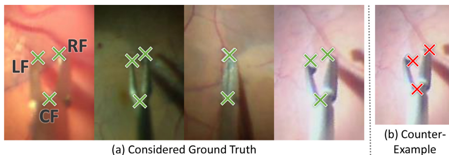
Fig. 3. Considered ground truth in instrument dataset: Due to the variation of instrument shapes, the ground truth has to be set in more detail in order to be well-defined. (a) shows examples for the considered ground truth. The tool tips (LF and RF) are set as the points on the tip which are closest to the microscope and would touch in case of a closed forceps. The center joint (CF) is the point connecting the two parts of the forceps. In (b), the annotation is not selected as the top visible part the tool tip points but on the part which is closer to the retina.
