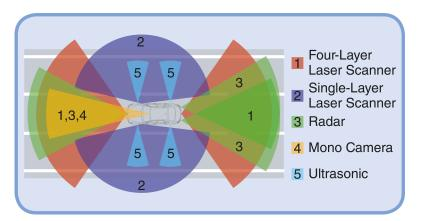
*Figure 6.* A possible sensor configuration of an automated vehicle illustrated by Aeberhard et al. (2015).
