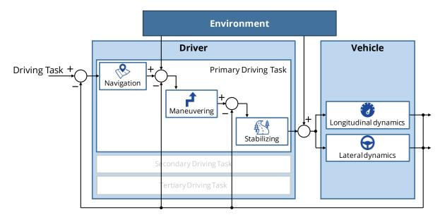
*Figure 3.* The driver-vehicle feedback loop; adapted from Bubb, Bengler, Grünen, and Vollrath (2015).
