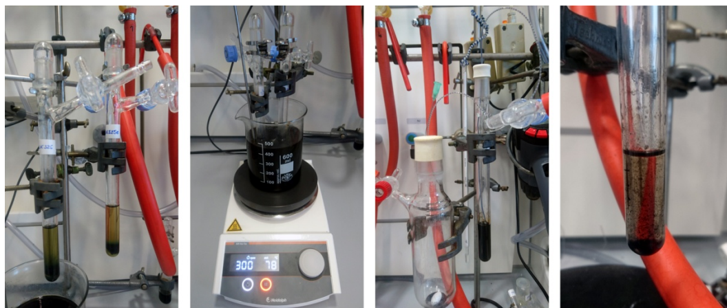
Figure 61. Preparative steps in the synthesis of [\text{Cu}_{43}(\text{AlCp}^*)_{12}] ( 3 ). The synthesis was always conducted in the depicted Schlenk flasks with a high surface to volume ratio (left, outer diameter: 1.3 cm). Starting reagents were weighed into the reaction vessel inside a glovebox. Freshly distilled benzene was added outside the GB, and the closed Schlenk flask was disconnected from the Schlenk line and placed in an oil bath which was pre-heated to 78^\circ\text{C} (middle left). After completed reaction and crystallization time, the product was isolated by slow and careful decantation using a narrow teflon cannula ( d < 1 mm; middle right). Repeated washing steps with benzene were performed analogously until the supernatant liquid remained colourless (right).
