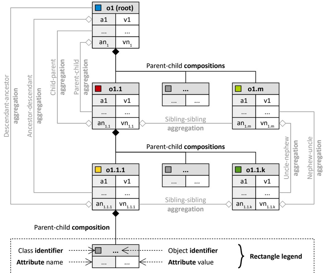
Figure 6.5: Hierarchical structure of the design objects with class and attribute annotations as well as cross references.
