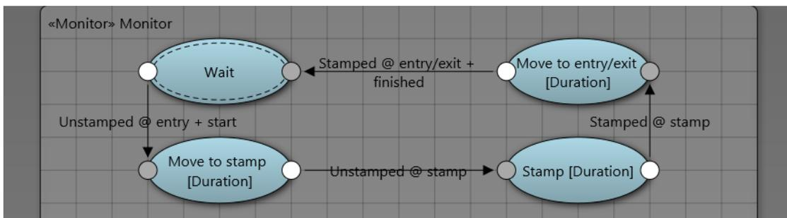
Figure 8.27: PPU stamper monitor view.
