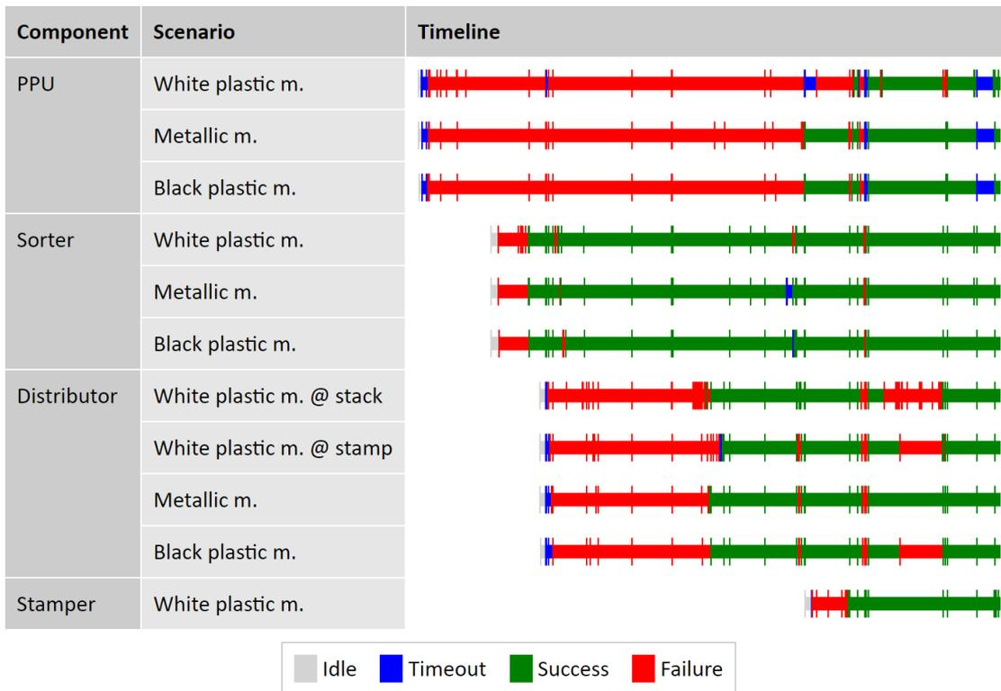
Figure 9.3: Test execution events and respective outcomes associated with the individual components and their scenarios over time.
