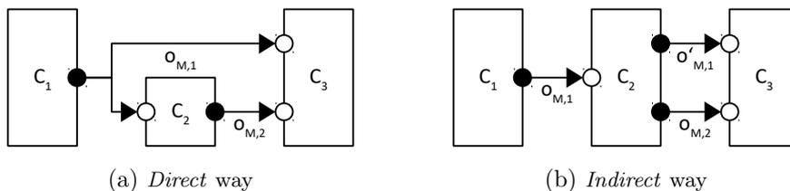
Figure 5.8: *Channel-based* model of kinematic chains.
