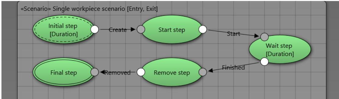
Figure 8.13: PPU single workpiece scenario view.
