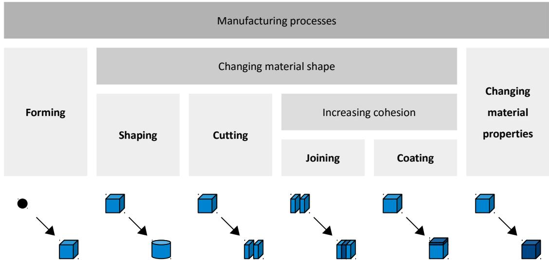
Figure 1.1: Production processes implemented by manufacturing systems [WW10].
