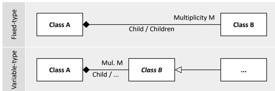
Figure 6.3: UML specification pattern for required fixed- or variable-type children.
