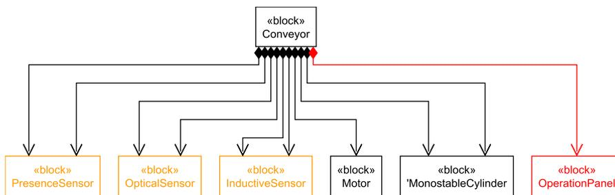
Figure 9.7: Component architecture of the conveyor module in the SysML documentation [LFVH13].
