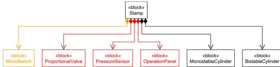
Figure 9.6: Component architecture of the stamp module in the SysML documentation [LFVH13].
