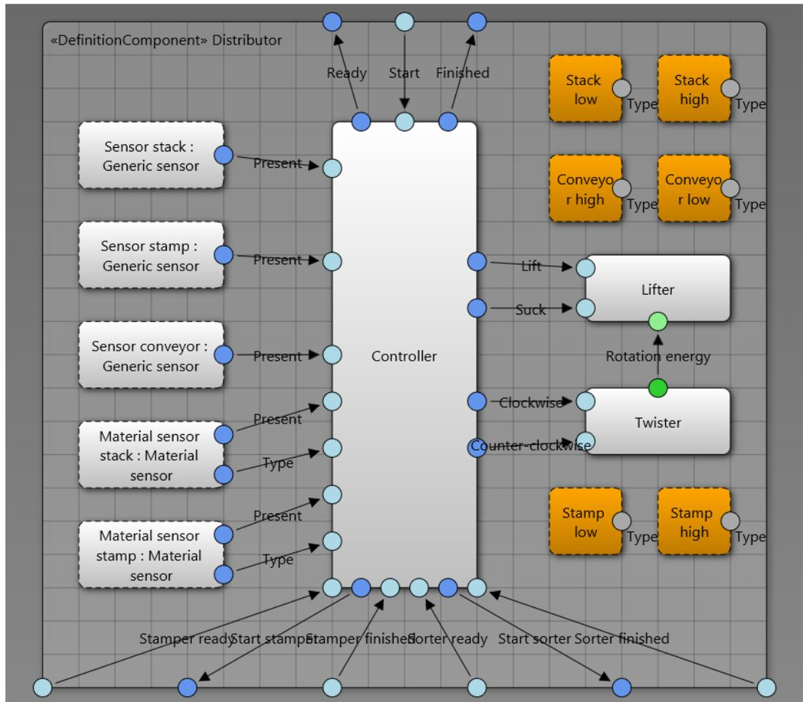
Figure 8.19: PPU distributor components/channels view.
