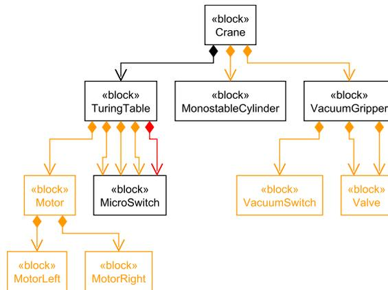
Figure 9.5: Component architecture of the crane module in the SysML documentation [LFVH13].
