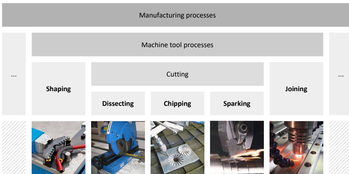
Figure 1.2: Production processes implemented by machine tools [Hir16].
