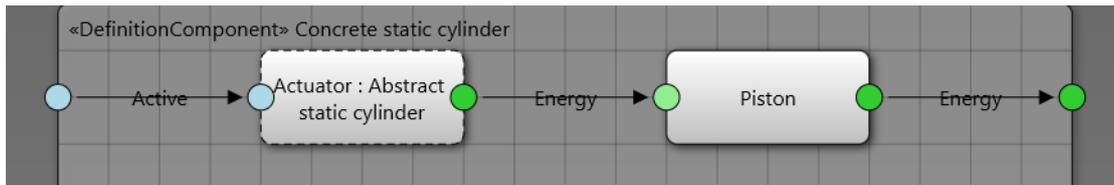
Figure 8.7: Concrete static cylinder components/channels view.
