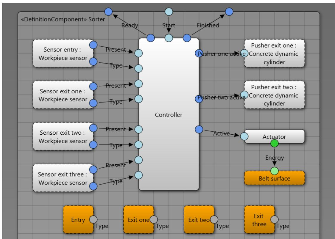
Figure 8.34: PPU sorter components/channels view.
