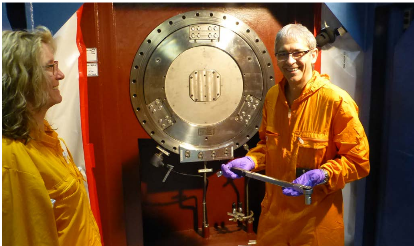
Figure 5: The new plug JMA16 is finally fixed on the beam tube SR6.
