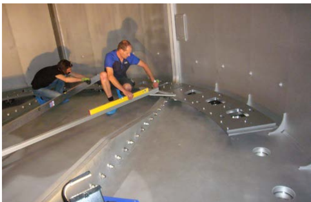
Figure 5: Inside the vacuum chamber the detector bank base plates were mounted and aligned with respect to the the sample center.
