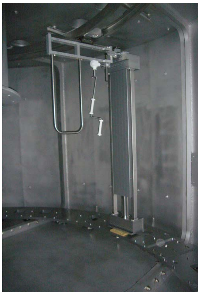
Figure 8: The detector box (for testing without tubes) is placed in the final position and mounted on the detector bank with the rail system and carriage.
