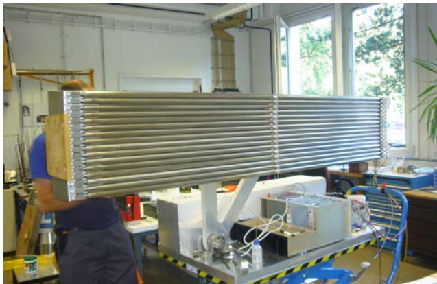
Figure 3: 16 detectors are mounted on a detector box.
