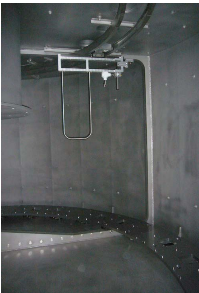
Figure 7: Assembly of the rail system with the carriage. Using this device, the detector boxes can be positioned and mounted inside the vacuum chamber.
