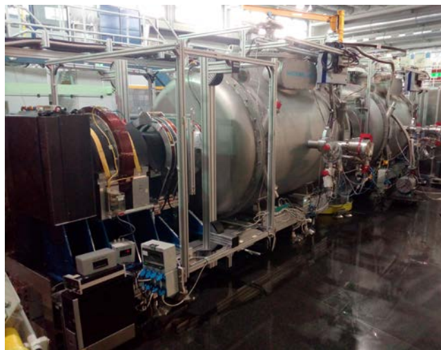
Figure 2: The new superconducting main precession coils in their cryostats in place at the J-NSE.
