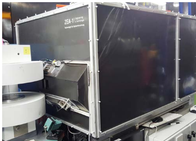
Figure 10: The closed and shielded cabinet in operation.
