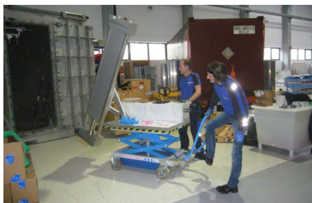
Figure 6: Trial installation of a detector box without He 3 detector tubes using a specially designed assembly cart.
