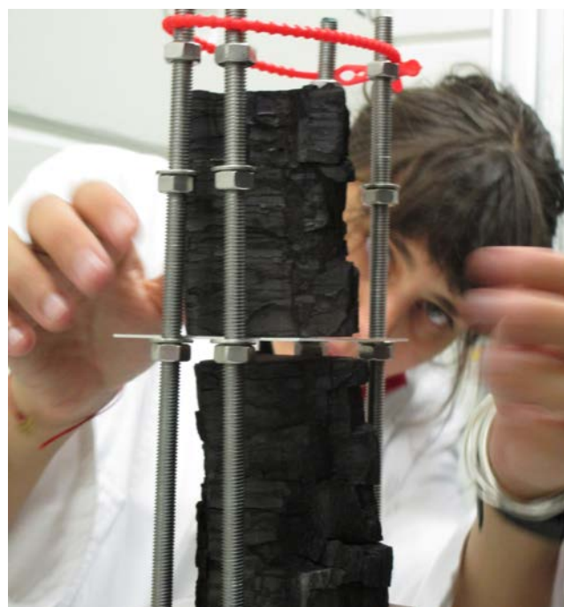
Figure 1: Experimental set-up for the neutron CT measurements at NECTAR.
