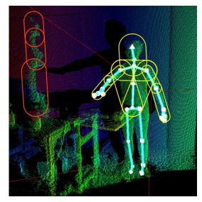
Fig. 4 Robot and human are each represented as a set of capsules for detection of the states "COLLISION POSSIBLE" or "COLLISION IMPOSSIBLE"
