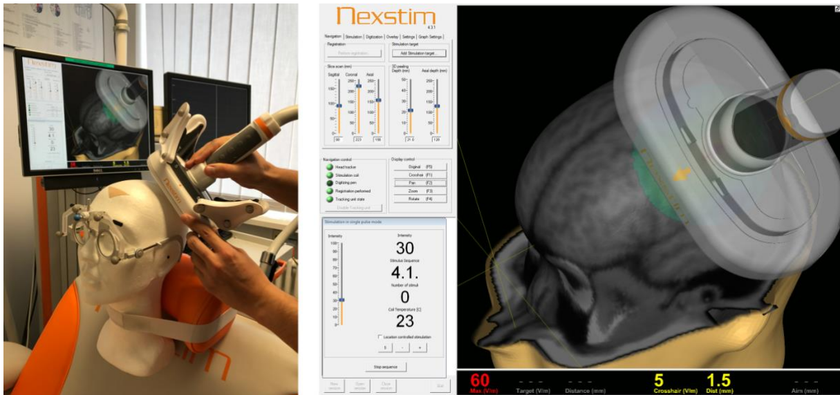
Fig. 11: Neuronavigation of the nTMS system; the head model represents the patient's head position; the patient is wearing glasses with tracking units, coil tracking units are also visible (left image); a camera (not in the picture) registers the position of the patient's head and the coil and superimposes the relative position of the coil on the 3D MRI sequence (right image)
