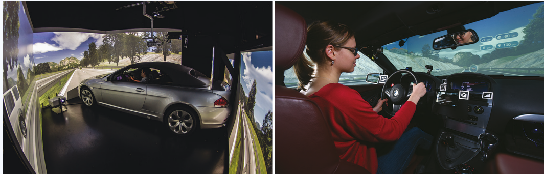
Figure 2.2: The driving-simulator setup with the cooperative interaction concepts under test. Photographers were Andreas Haslbeck (exterior, 2015) and Tobias Hase (interior, 2016).
