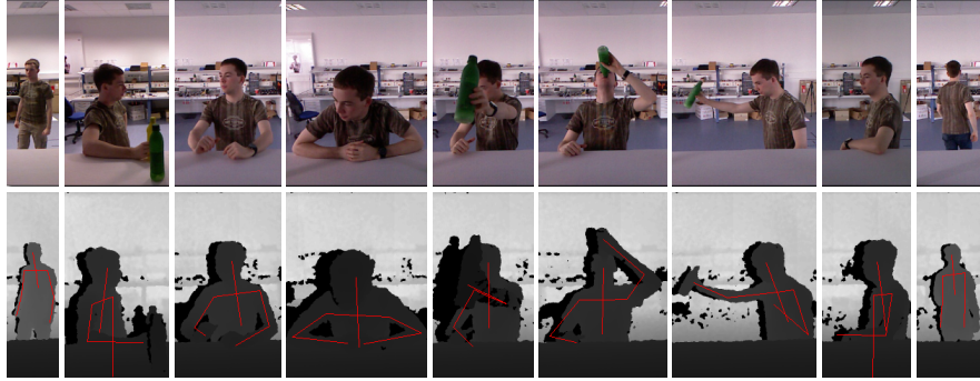
Fig. 14 Camera images (top) and corresponding skeleton poses (bottom) of Kinect sensor used for visual intention recognition. The recognized states in the bar scenario include (from left to right): entering bar setting, leaning on bar with right side, requesting attention, raising glass with left hand, drinking, raising glass with right hand, leaning on bar with left side, and leaving bar setting.
