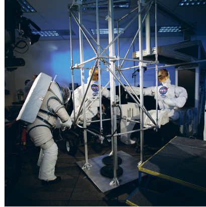
Fig. 4 Multiple Robonaut humanoids in a joint construction task (Copyright NASA).
