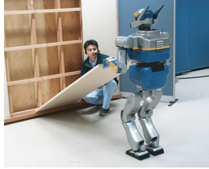
Fig. 6 HRP-2 humanoid working together with a human in the construction of a cottage [35].
