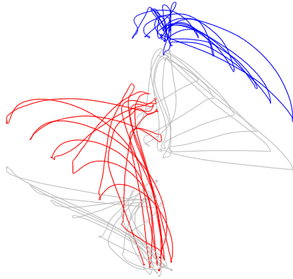
Fig. 2a 3D plot of human-human interaction in the handover experiment. The giving subject ( top, blue ) hands over six cubes to the receiver ( bottom, red ). The projection of the movements on the table surface is shown in gray .
