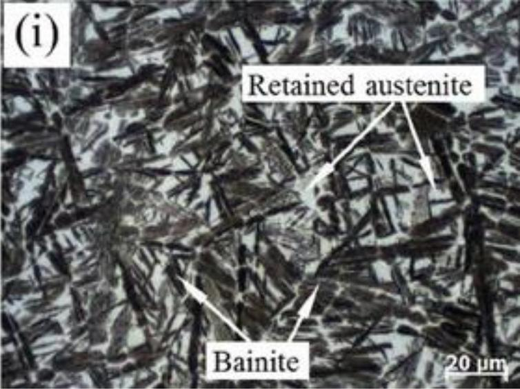
**Figure 1.5** Optical micrographs of bainite obtained at 200 °C [Yguo15].
