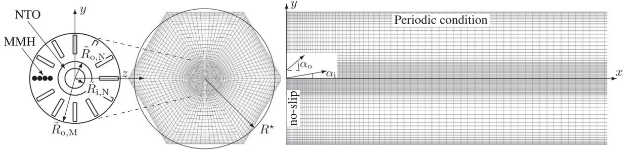
**Figure 1.** MMH and NTO injection (left), numerical grids in y-z plane (middle), and upstream part of the grid in the x-y plane (right). Injection angles of NTO at  $\tilde{R}_{i,N}$  and  $\tilde{R}_{o,N}$  (right). MMH: monomethylhydrazine; NTO: nitrogen tetroxide.
