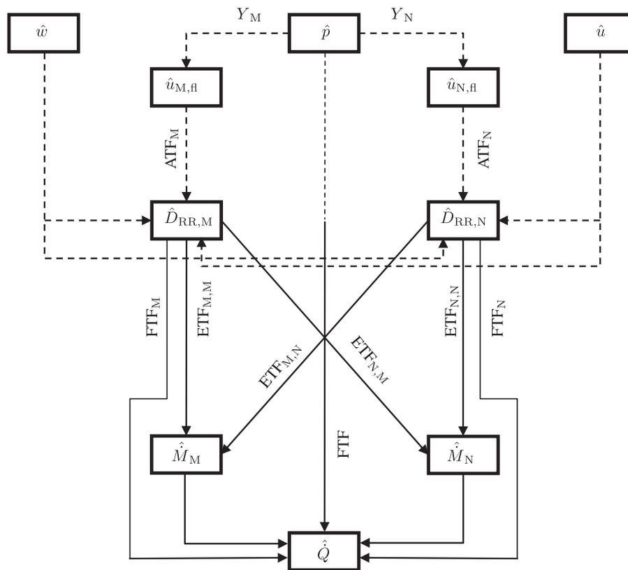
**Figure 5.** Influence of acoustic fields in hypergolic rocket engines on atomization quality, evaporation, and dynamic heat release in the flame. FTF: flame transfer function; ETF: evaporation transfer function; ATF: atomization transfer function.
