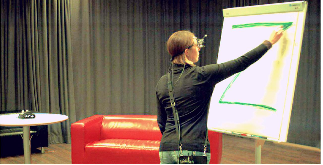
Figure 5: A human participant repetitively draws large “Z” letters on a flip chart, while naturally tracking the pen with the eye. The human gaze motion is captured in workspace coordinates using a combination of eye tracking and marker based head motion tracking.
