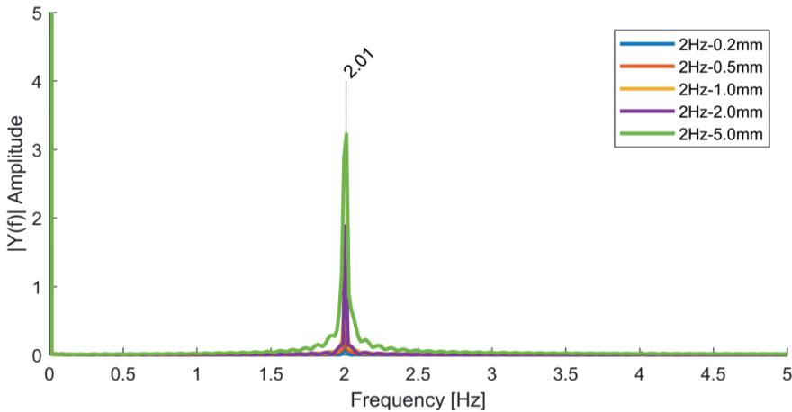
Fig. 4 Frequency spectrum of analysed experiments with varying amplitudes
