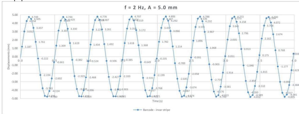
Fig. 3 Detail (first 4 seconds) of one analysed video stream; every dot represents the vertical displacement of one video frame
