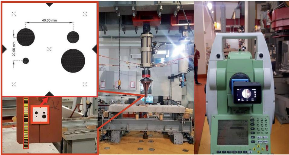
*Fig. 2 Signal marks-barcode and photomark (red on the left), testing machine (middle) and IATS prototype (right)*
