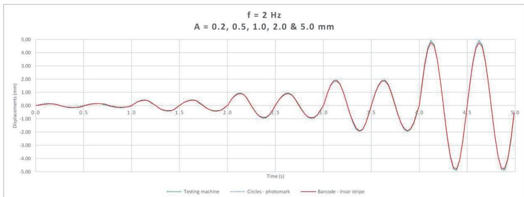
Fig. 5 Resulting amplitudes of five different experiments (1 sec period each experiment)
