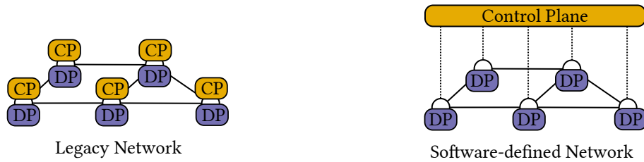
(a) Legacy network where the control plane (CP) and the data plane (DP) are integrated into a device.
