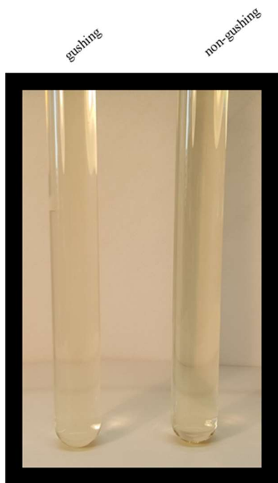
Figure 7: sparkling wines in test tubes, left: gushing sparkling wine with modified light scattering properties, right: non-gushing sparkling wine as negative control
