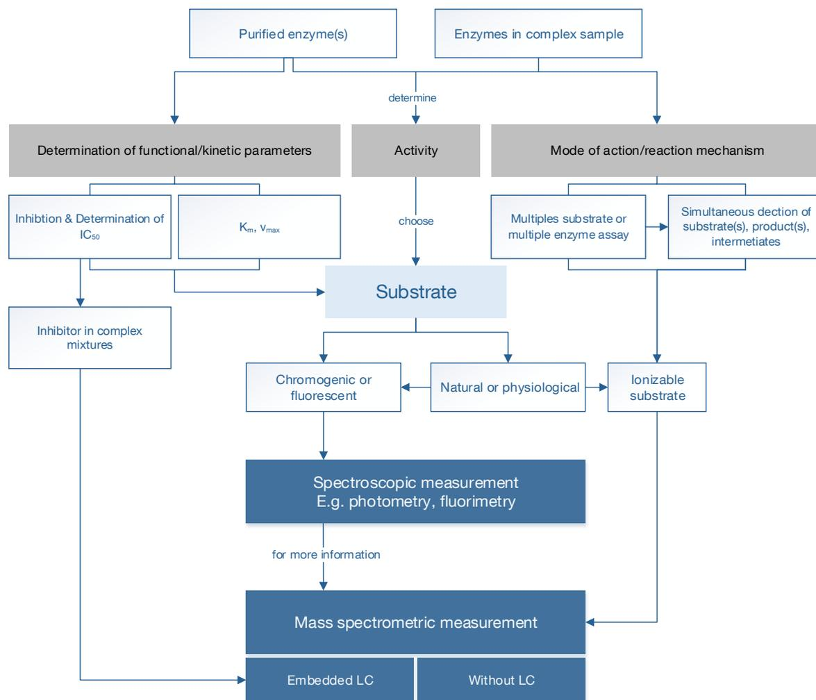
Figure 2-3: Selection pathway to choose an appropriate detection method for measuring enzymatic reactions.
