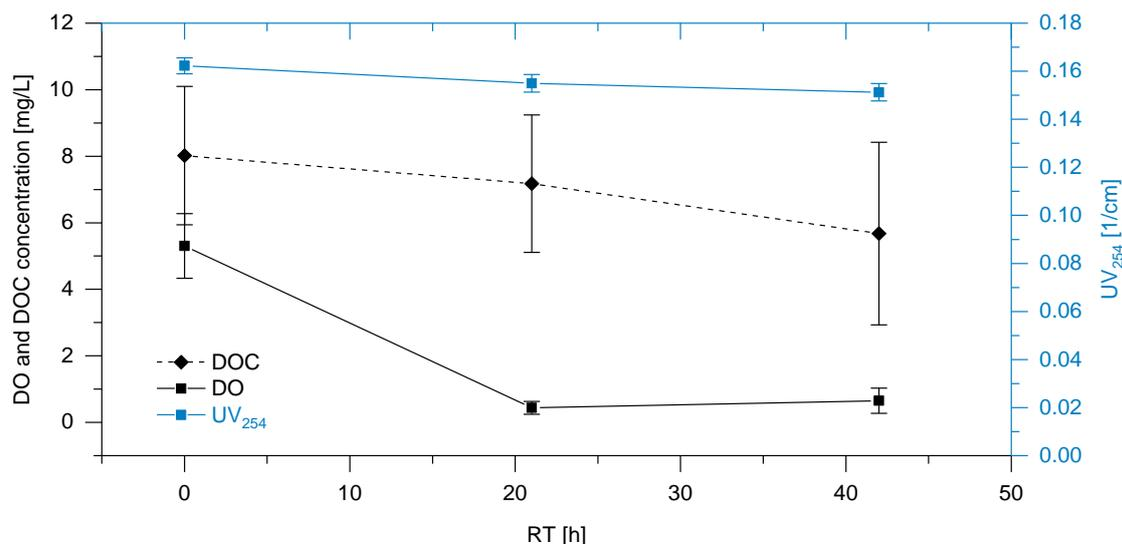
Figure 5-1: Concentration [mg/L] of dissolved organic carbon (DOC) and dissolved oxygen (DO) as well as the absorption coefficient at 254 nm ( $UV_{254}$ ) [1/cm] in the influent and effluent of the first and second column of the soil-column system,  $n \geq 3$ .
