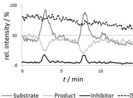
**Figure 6.** Online coupled xanthine oxidase bioassay after a double injection of the known inhibitor allopurinol. The uric acid product trace decreases and the xanthine substrate trace increases when allopurinol is present. IS is the internal standard.
