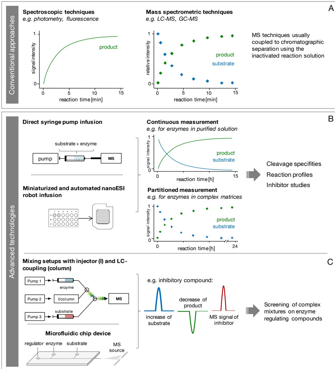
Figure 2-2: Overview of techniques for studying enzymatic reactions. Basic approaches, miniaturization, and resulting data are shown schematically for (A) conventional approaches, (B) syringe pump assay and (C) the online coupled continuous flow setup. Adapted from Burkhardt et al. (2015), see Appendix I.
