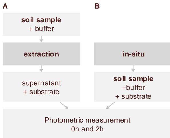
Figure 1: Scheme of (A), extraction, and (B), in-situ approach.
