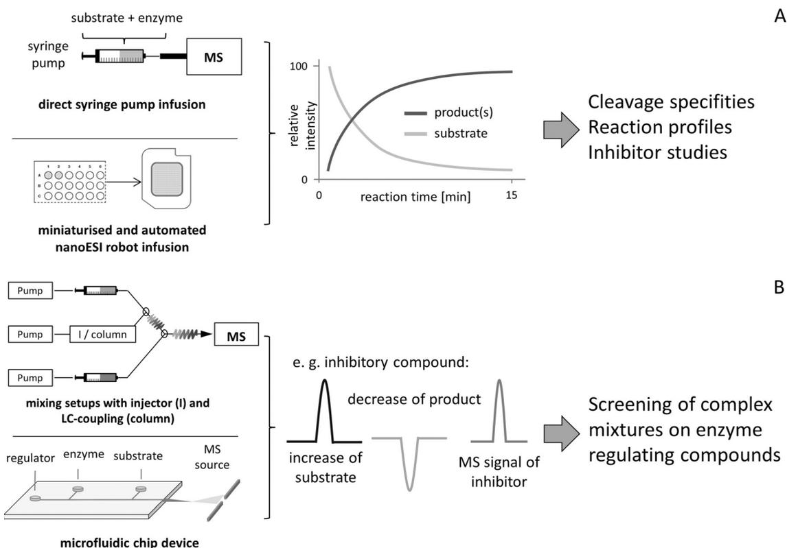
**Figure 1.** Overview of coupling techniques for studying enzymatic reactions by continuous-flow measurements. Basic approaches, miniaturization, and resulting data are shown schematically for A) a syringe pump assay, and B) the online coupled continuous-flow setup. Adapted from R. K. Scheerle, PhD thesis, TU München.
