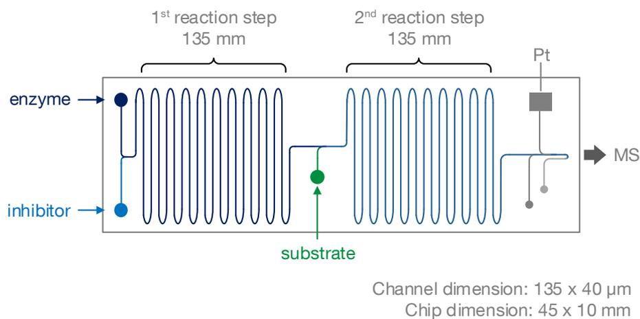
Figure 7-1: Final layout and dimensions of the microfluidic chip. Adapted from AG Belder (Leipzig).
