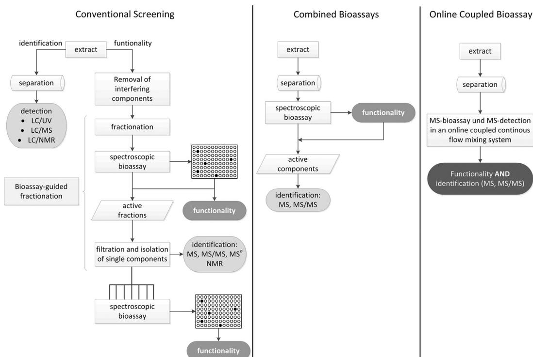
**Figure 5.** Workflow comparison for three different methodological approaches with regard to the assessment of functional bioassays.
