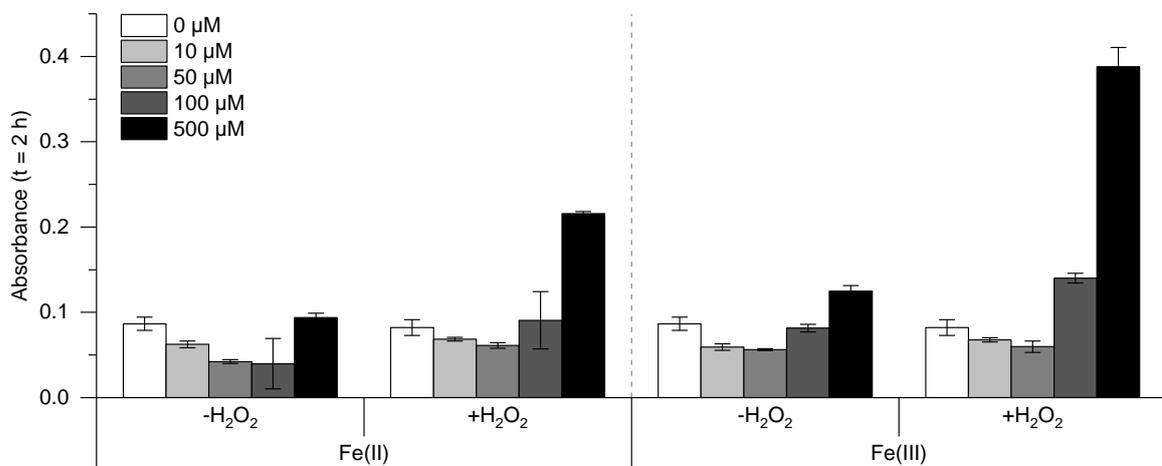
Figure II: Substrate oxidation in the presence of 0  $\mu M$ , 10  $\mu M$ , 50  $\mu M$ , 100  $\mu M$ , and 500  $\mu M$  Fe(II) or Fe(III) in absence of samples from MAR systems using pyrogallol as substrate. Assays were conducted in the absence ( $-H_2O_2$ ) and presence ( $+H_2O_2$ ) of hydrogen peroxide at pH 7.0. Mean values  $\pm$  standard deviation ( $n = 3$ ) are shown.
