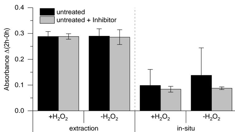
Figure 3: Substrate oxidation of untreated and autoclaved samples from MAR systems with 0.1 mM sodium azide (SAz). Shown is a difference in absorbance  $\Delta(2h-0h)$  for extraction and in-situ method using pyrogallol (PYR) as a substrate. Assays were conducted in the absence ( $-H_2O_2$ ) and presence of hydrogen peroxide ( $+H_2O_2$ ) at pH 7.0. Mean values  $\pm$  standard deviation ( $n \geq 3$ ) are shown.
