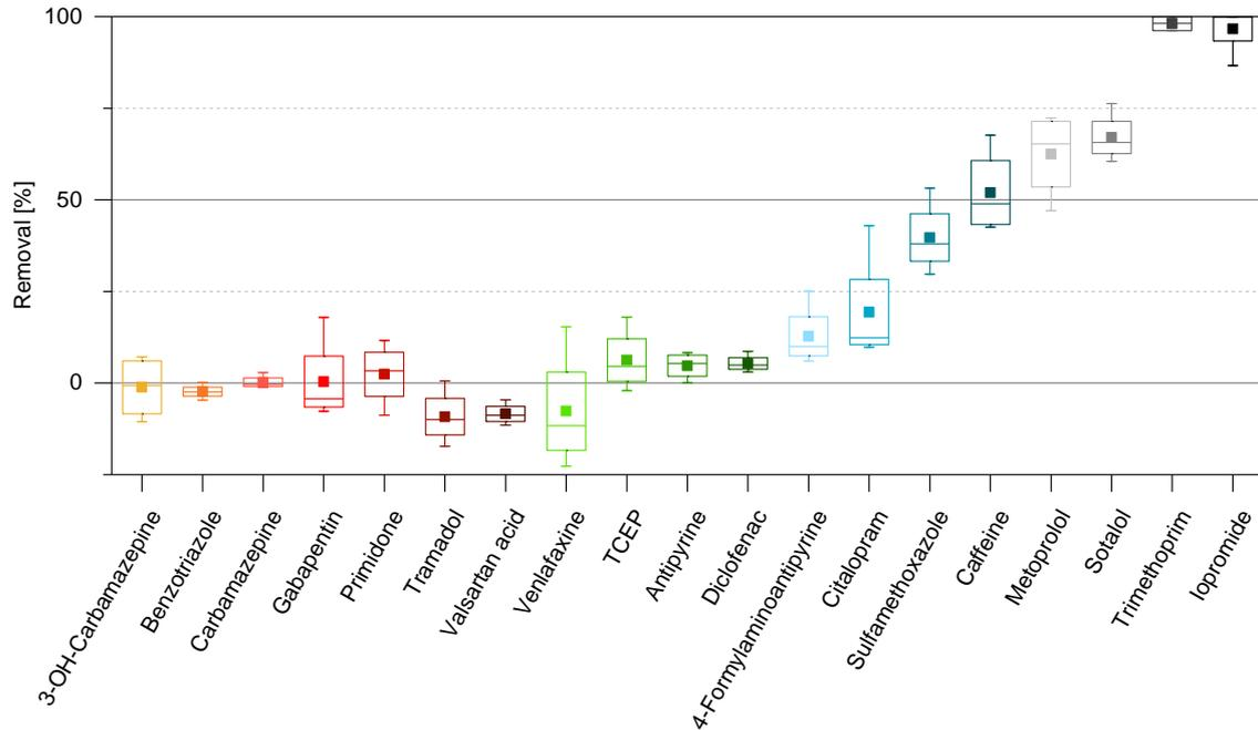
Figure 5-2: Removal of selected trace organic chemicals (TOrcs) in soil-column setup after 42 h,  $n \geq 4$ .
