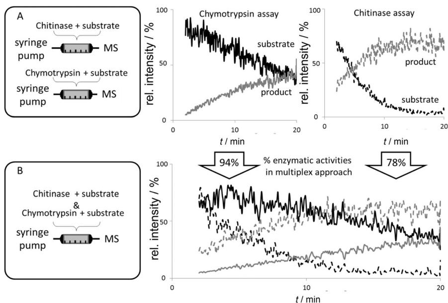
**Figure 3.** Direct syringe pump infusion assay with the enzymes chitinase and chymotrypsin. A) Individual enzymatic reactions of chitinase and chymotrypsin in the presence of their corresponding substrates, in comparison with B) the multiplex approach, in which both enzymes were measured simultaneously in one assay.
