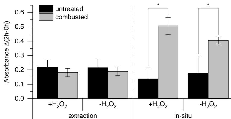
Figure 4: Combustion experiments with untreated samples from MAR systems. Substrate oxidation of the untreated and untreated/combusted sample are shown as difference in absorbance  $\Delta(2h-0h)$  for extraction and in-situ method using the pyrogallol (PYR) as a substrate. Assays were conducted in the absence ( $-H_2O_2$ ) and presence ( $+H_2O_2$ ) of hydrogen peroxide at pH 7.0. Mean values  $\pm$  standard deviation ( $n \geq 3$ ) are shown.
