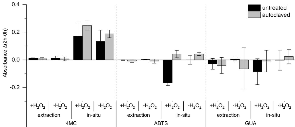
Figure I: Substrate oxidation of the untreated sample and autoclaved (20 min, 121 °C) samples from MAR systems shown as difference in absorbance  $\Delta(2h-0h)$  for extraction and in-situ methods using 4-methylcatechol (4MC), ABTS, and guaiacol (GUA) as the substrate. Assays were conducted in absence ( $-H_2O_2$ ) and presence ( $+H_2O_2$ ) of hydrogen peroxide at pH 7.0. Mean values  $\pm$  standard deviation ( $n \geq 3$ ) are shown.
