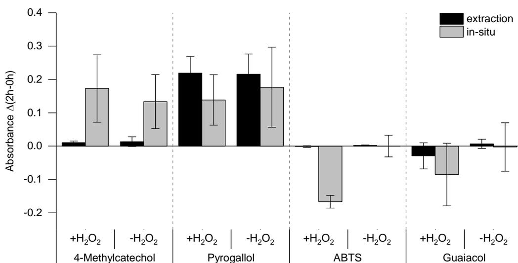
Figure 2: Substrate oxidation in samples from MAR systems with different substrates. Shown is the difference in absorbance  $\Delta(2 h-0 h)$  for the extraction and in-situ method using ABTS, guaiacol (GUA), 4-methylcatechol (4MC), and pyrogallol (PYR). Assays were conducted in the absence ( $-H_2O_2$ ) or presence of hydrogen peroxide ( $+H_2O_2$ ) at pH 7.0. Shown are mean values  $\pm$  standard deviation ( $n \geq 3$ ).
