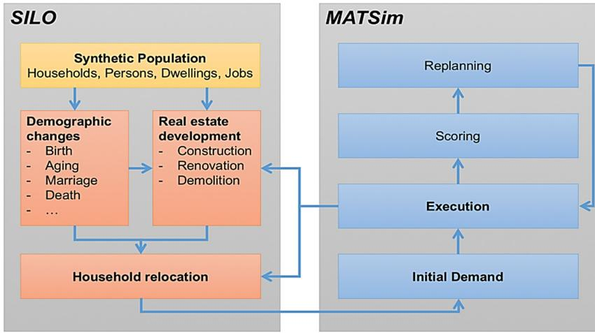
Figure 3: Integration of the land use model SILO with the transport model MATSim
