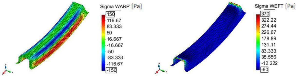
Fig. 9 30° rib: 0°/90° ply - warp-stress (left) and weft-stress(right)
