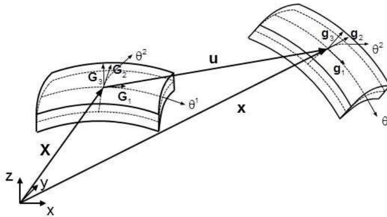
Fig. 1. Nonlinear kinematics of thin membrane structures.
