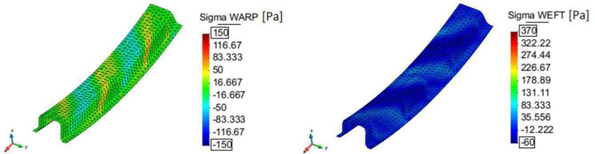
Fig. 10 Figure 24: 30° rib: 45°/-45° ply - warp-stress (left) and weft-stress(right)
