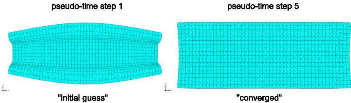
Fig. 6. 30° rib: Initial guess (left) vs. optimized cutting pattern (right)
