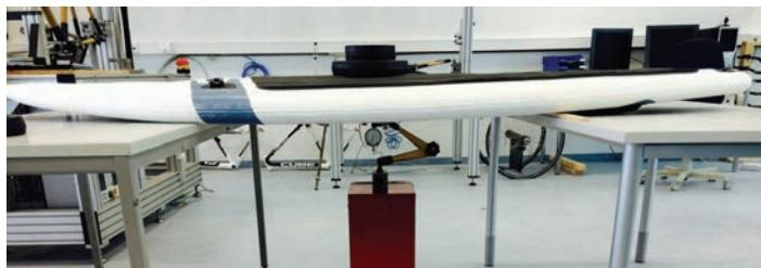
Fig. 5. Three-point-bending test (above: Dropstitch, below: VacuuAir)
