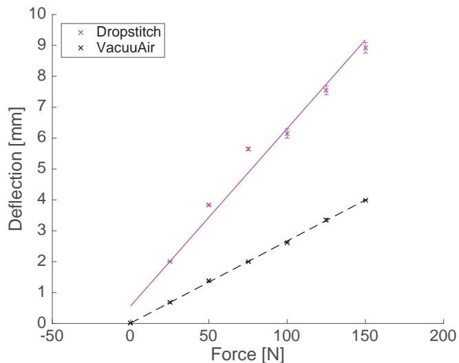
Fig. 6. Deflection as function of the applied force
