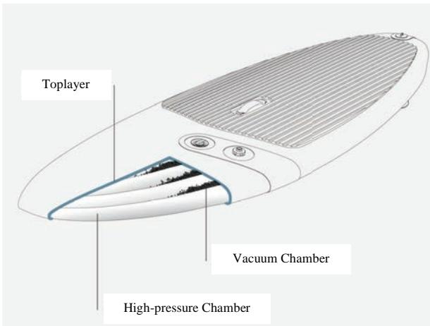
Fig. 3. VacuuAir-construction: chamber arrangement
