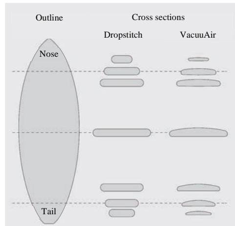
Fig. 4. Shape comparison of Dropstitch and VacuuAir
