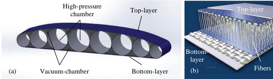
Fig. 2. (a) VacuuAir-construction; (b) Dropstitch-construction [4]
