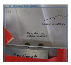
Figure 4.8.: CR-39 detector (outline marked in blue, numbered with '144') irradiated at  $50\,k\text{Vp}$  and  $70\,m\text{A}$  at a rotating anode X-ray tube for over  $10\,h$ . Two absorbers, a piece of tungsten alloy in the lower part and a  $200\,\mu\text{m}$  thick tungsten wire were placed in front of the CR-39 to generate transitions from irradiated to non-irradiated regions.
