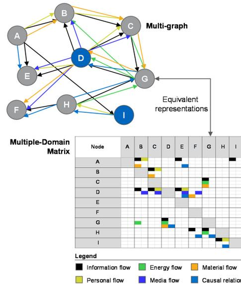
Fig. 1. Multi-graph and Engineering Systems Multiple-Domain Matrix
