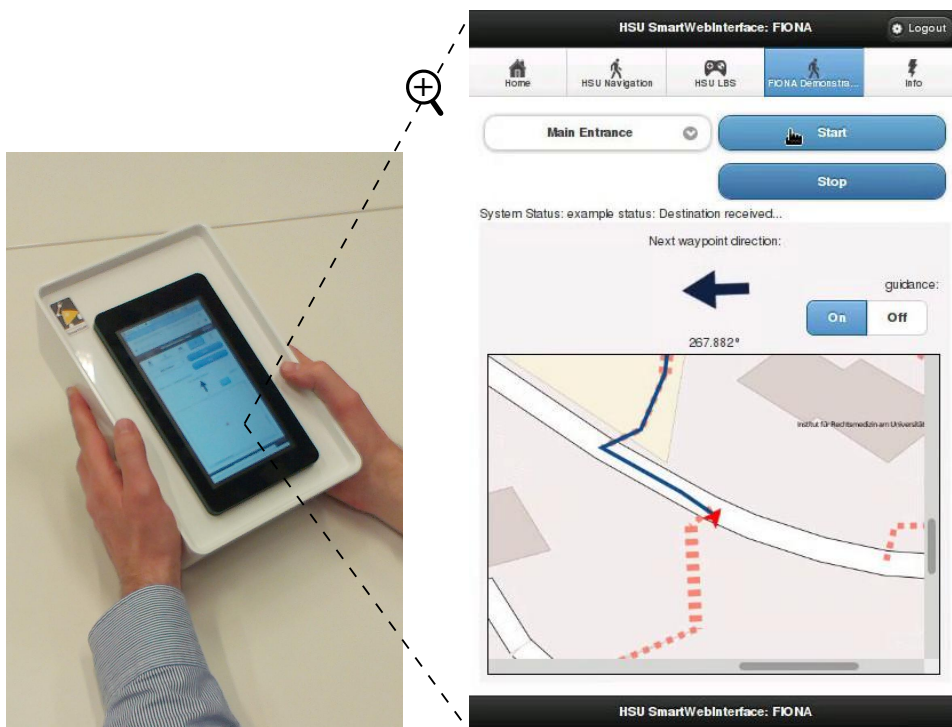
Figure 7.6: The Personal Mobile Navigation Demonstrator: the handheld device (left) and its graphical user interface (right). Video at [SF16].
