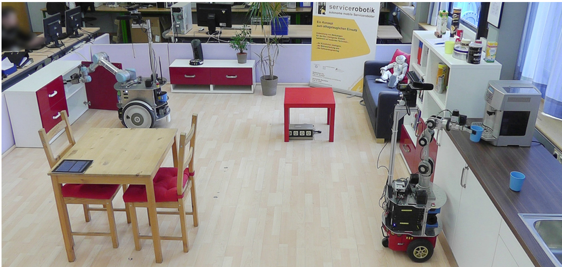
(a) The service robots Larry (left) and Kate (right). Larry grasps an object after opening the door of the cupboard. Kate operates the coffee machine.
