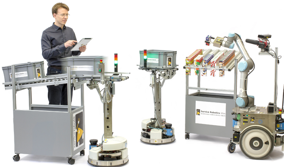
Figure 7.11: The “Industry 4.0 Robot Commissioning Fleet in Intra-Logistics” scenario. Three robots feature: navigation in a robot fleet, mobile manipulation for order picking, and handling of boxes. Video at [Lut+17].
