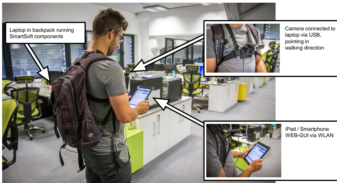
Figure 7.8: The “ Visual Localization Demonstrator ” for personal navigation in an office space. Video at [SFC15].
