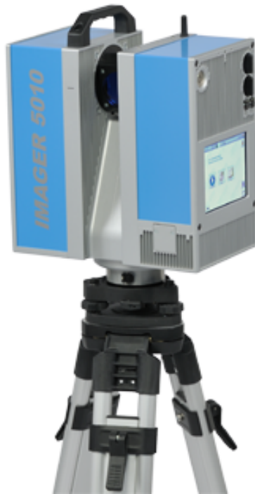
Figure 3.9: The Zoller & Fröhlich 5010C laser scanner used to generate the dataset. Image retrieved from http://www.zf-laser.com
