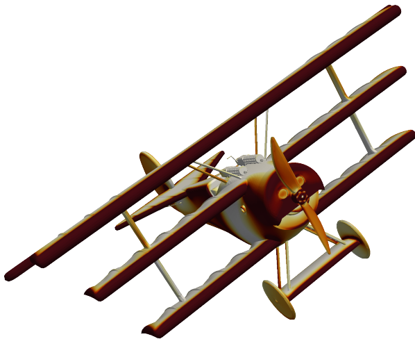
Fig. 8.10.: Fokker Dr.I: real part of j excited by an incident plane wave.
