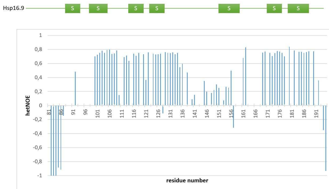
Figure 16: Heteronuclear NOE spectrum of the truncation mutant Hsp26 \alpha M1. A protein concentration of 0.1 mM was used. A decrease in signal intensities is observed for the residues 135-155. Structured elements of the respective wheat Hsp16.9 residues are indicated in green. Figure provided by Dr. Hyun-Seo Kang (Chair for biomolecular NMR spectroscopy, TUM).
