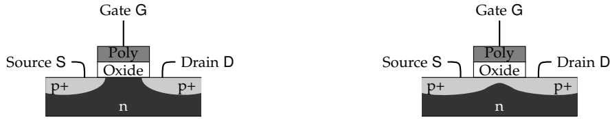
(a) If V_{GD} \geq V_T , then the two regions p+ are isolated and the pMOS is turned "OFF". (b) If V_{GD} < V_T , then a channel is created between the two regions p+ and the pMOS is turned "ON".
